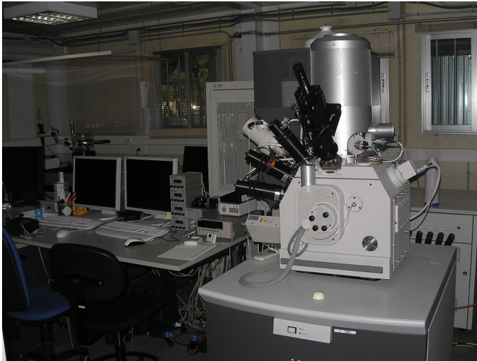
FEI Nanolab 200 Dual beam (SEM + FIB) in operation at INA
