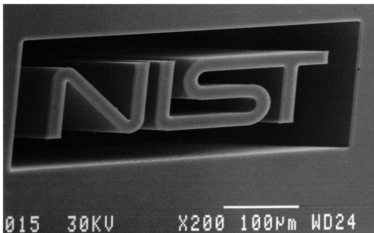
Figure 16: Electron micrograph of a test structure etched using DRIE, demonstrating the arbitrary geometries possible with this technique.
